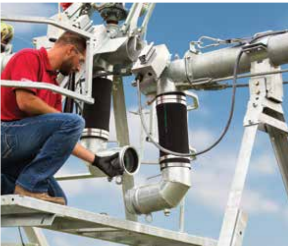
Full 6 5/8 in. diameter hose connection
